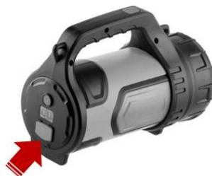
To charge the lamp, open the cover on the back of the lamp and plug the lamp into a charging device using the cable provided.
