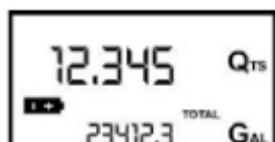
When the battery charge falls below the first level on the lcd, the fixed battery symbol appears.
