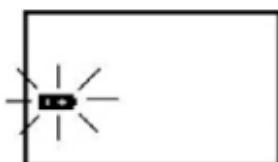
When the battery charge is no longer sufficient and prevents the digital counter from operating. The battery icon flashes.
