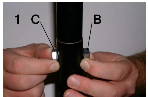
Join the full push bar to frame F (see photo 2 and fig. 1). Mount washer E and locknut D.
