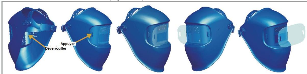
Refit the new screen, ensuring that it is correctly held by the two tabs.
