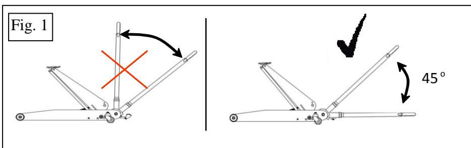
Please Note! The pump handle may only be used pumping, from an angle of  $45^{\circ}$  and down. This is done to prevent damaging the pump and to achieve the most ergonomically correct way of working.
